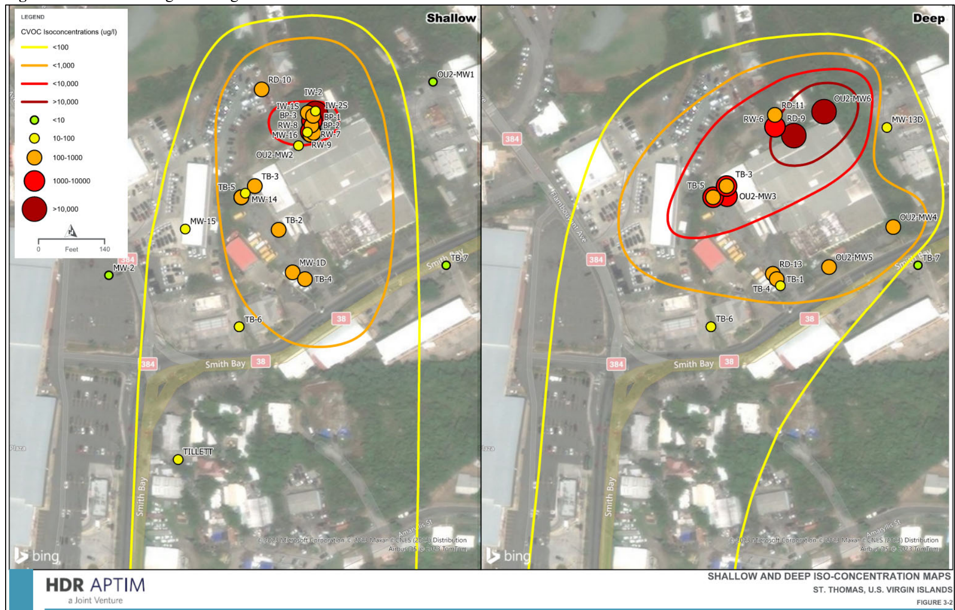
Figure 5: 2023 Pre-Design Investigation Plume Extent
