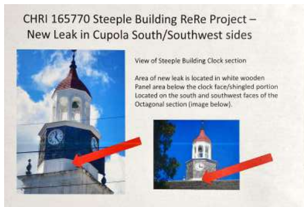
FIGURE 2-63. Photographs taken in 2017 by the National Park Service staff showing the location of a newly identified leak in the cupola. Source: National Park Service, Christiansted National Archives.
