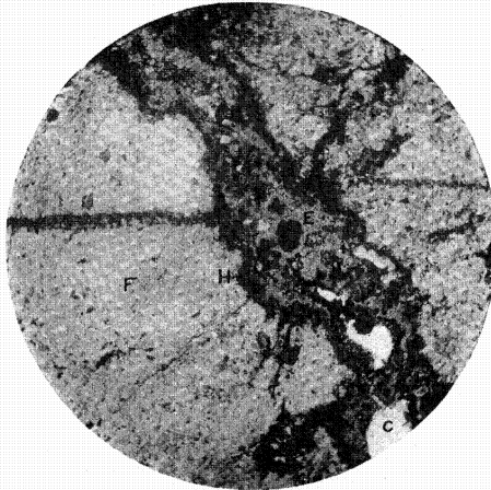
FIG. 21.— Latite, showing veins filled with epidote and iron oxides
