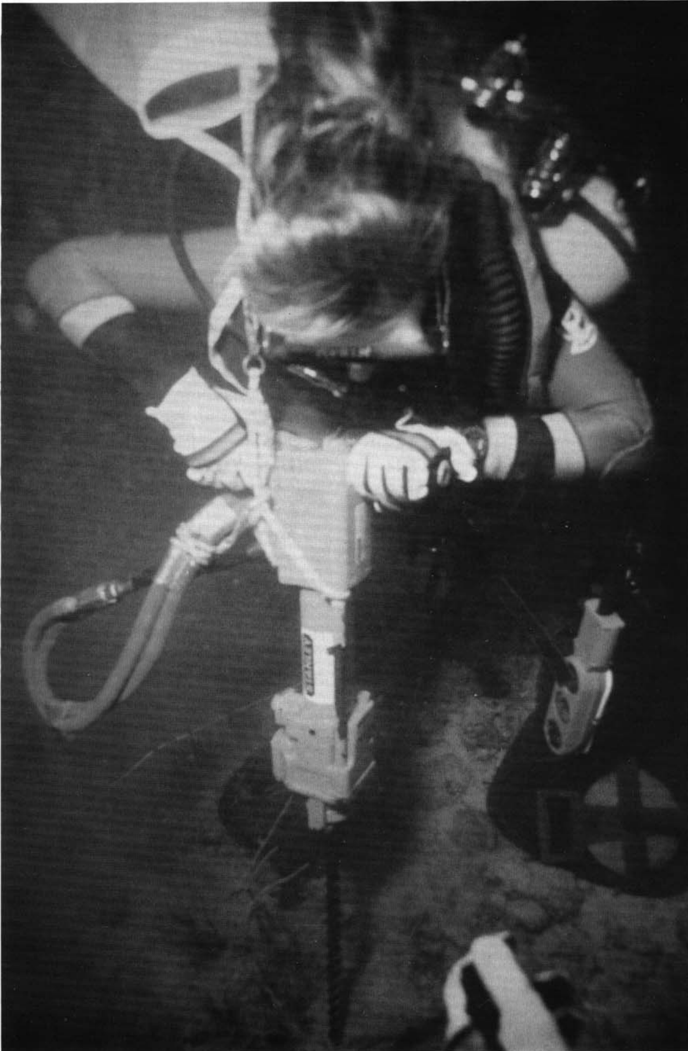
A diver uses a Stanley hydraulic impact-twist drill operated by a 15-hp. hydraulic supply from the surface to provide a hole for a permanent stake.
