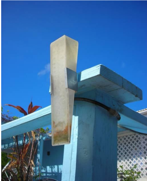
Rain gauge used to measure daily rainfall at Fish Bay. Recently installed sediment trap at Caribe Road.
