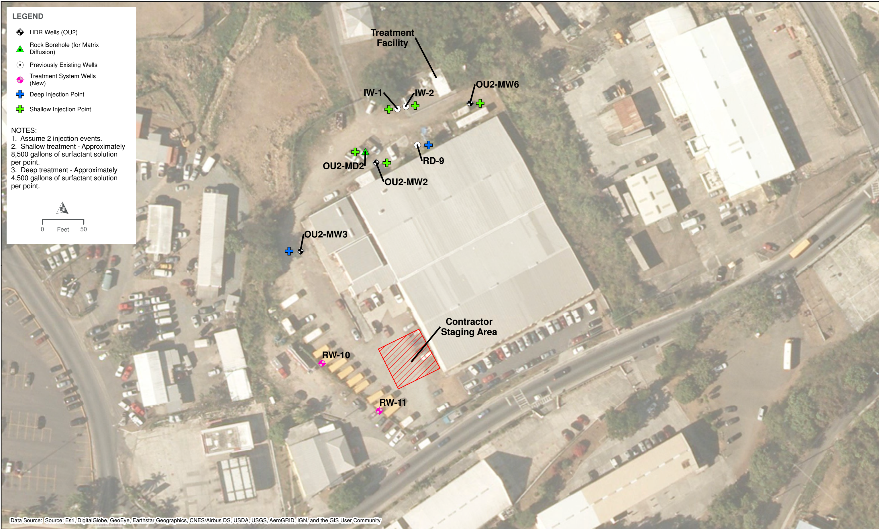
ALTERNATIVE 2D - EXPANSION OF PUMP AND TREAT SYSTEM AND SURFACTANT FLUSHING TUTU OU2, ST. THOMAS, U.S. VIRGIN ISLANDS
