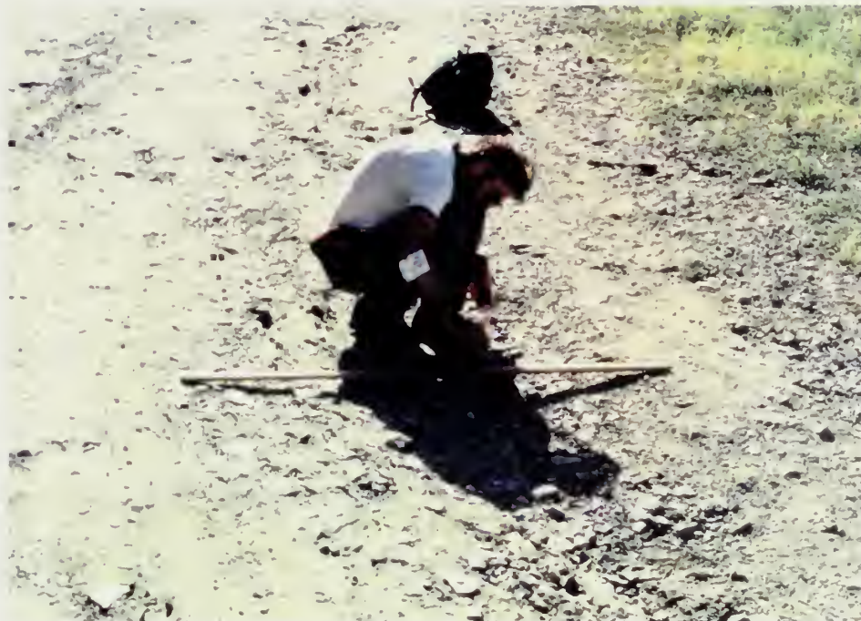
Figure 4.4. Measurement of cross-sectional road erosion.
