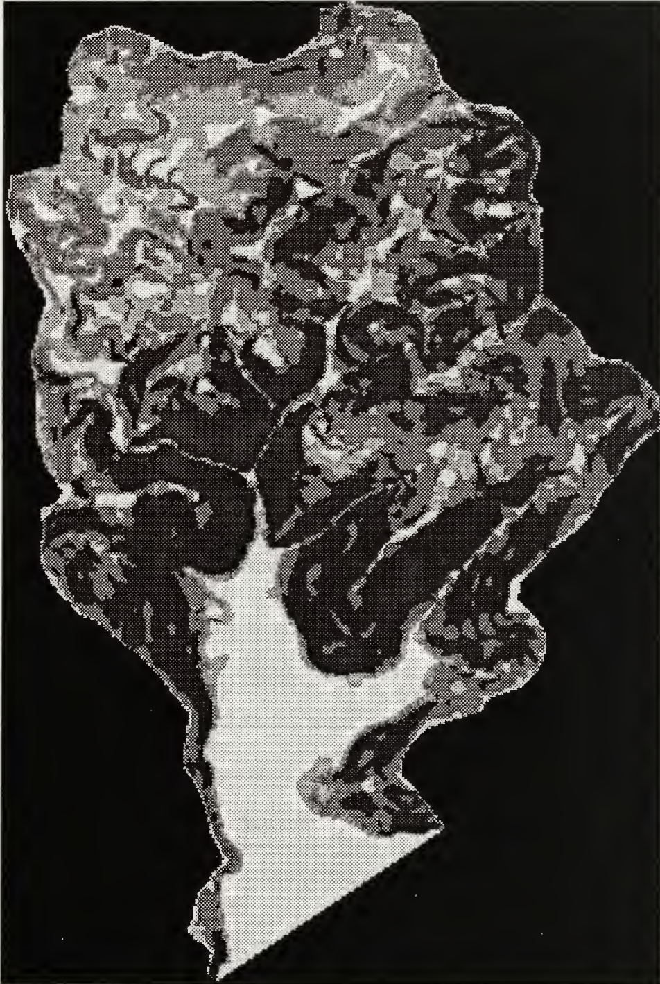
Figure 6.2. Calculated slope gradients in Fish Bay watershed. Lightest to darkest grid cells respectively represent 0-10%, 10-20%, 20-40%, and greater than 40% slope gradients.
