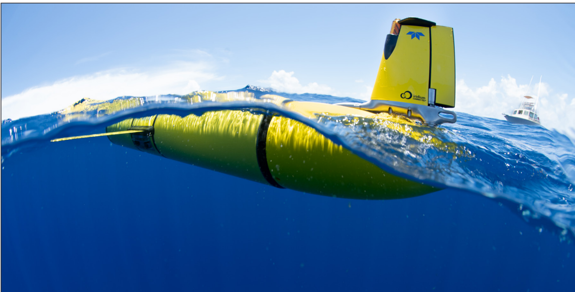
One of the new and exciting advances in oceanographic monitoring equipment is taking place in the arena of ocean glider technology. Ocean gliders are a type of autonomous underwater vehicle. These unmanned remote-controlled ocean gliders provide real-time data on ocean temperatures, salinity, dissolved carbon and many other ocean properties across a depth range from the surface to 3,000 feet underwater. The Slocum glider seen here was launched by Ocean and Coastal Observing Virgin Islands as part of a project to better understand hurricane intensification.
